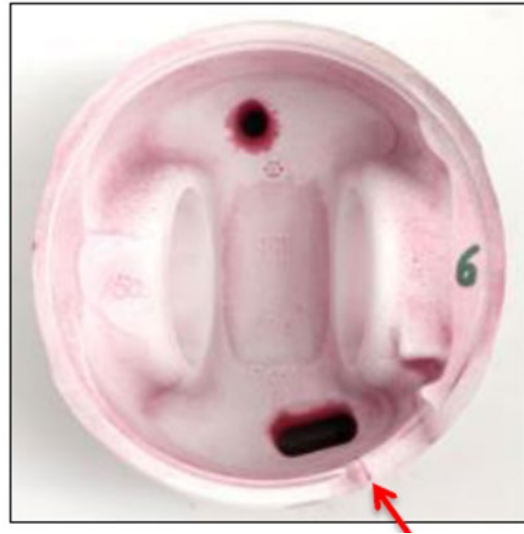
Figure 3. Piston bottom view – crack revealed (dye penetrant examination)
