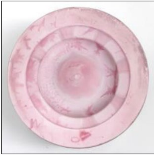
Figure 2. Piston crown – top view (no issues observed)
